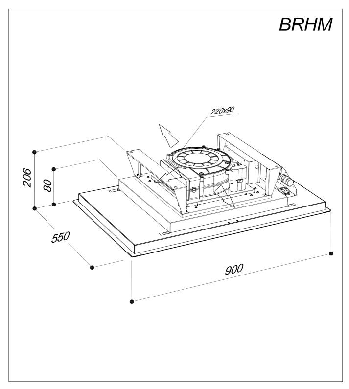
For the installation, create a false ceiling with a niche of 865mm for 515mm whose minimum height to be reached is 210mm
