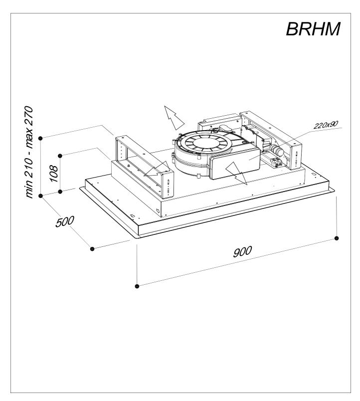
For the installation, create a false ceiling with a niche of 865mm for 465mm whose minimum height to be reached is 210mm
