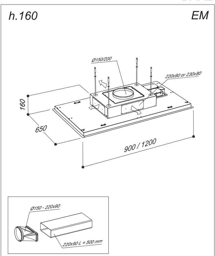
For the installation, create a false ceiling with a niche of 1165mm for 615mm whose minimum height to be reached is 170mm
