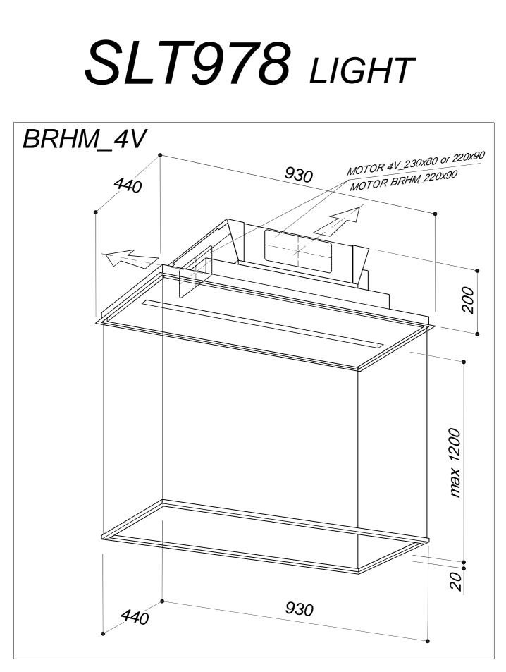
For the installation, create a false ceiling with a niche of 915mm for 425mm whose minimum height to be reached is 200mm
