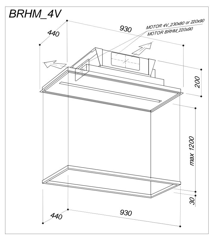
For the installation, create a false ceiling with a niche of 915mm for 425mm whose minimum height to be reached is 200mm
