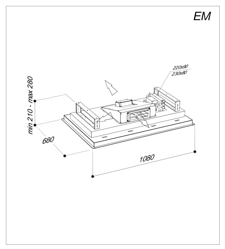
For the installation, create a false ceiling with a niche of 1050mm for 645mm whose minimum height to be reached is 210mm
