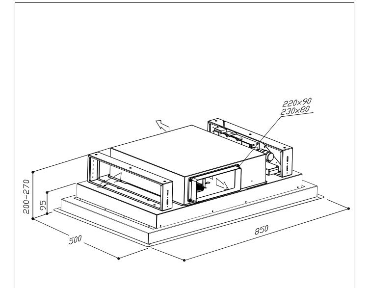
For the installation, create a false ceiling with a niche of 815mm for 465mm whose minimum height to be reached is 200mm
