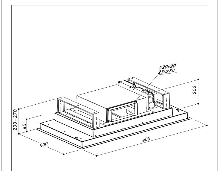
For the installation, create a false ceiling with a niche of 865mm for 465mm whose minimum height to be reached is 200mm
