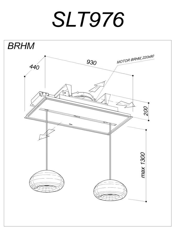
For the installation, create a false ceiling with a niche of 915mm for 425mm whose minimum height to be reached is 200mm
