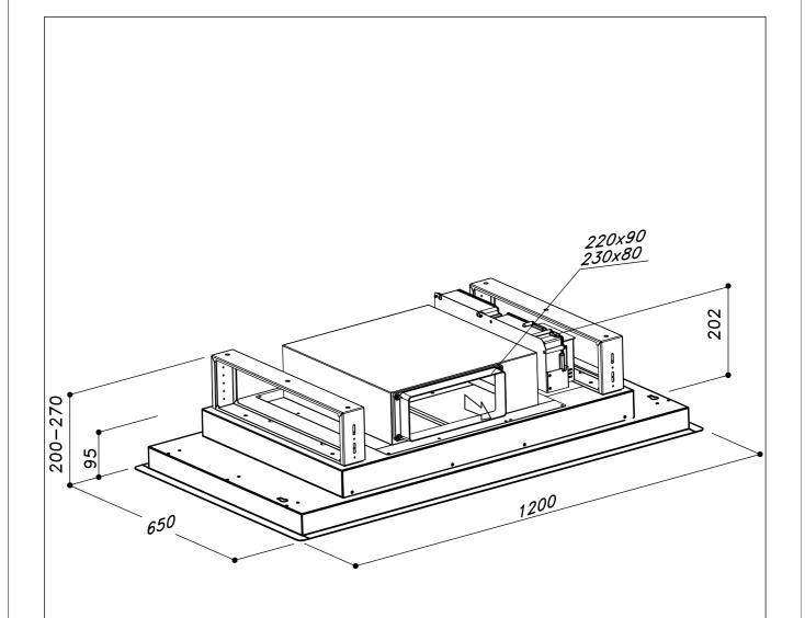
For the installation, create a false ceiling with a niche of 1165mm for 615mm whose minimum height to be reached is 200mm
